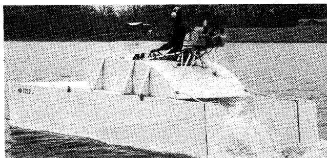
Fig. 5 FICAT II at speed on calm water. As the first manned supercritical ships, the FICAT's demonstrated the practicality of the concept under the scaled "real world" conditions in the Chesapeake Bay.
